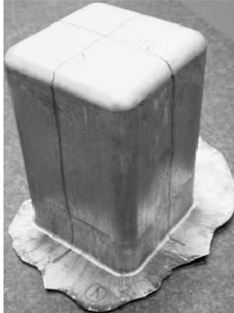
Figure 4.23: Warm deep drawn square cup (courtesy Corus RD & T).
